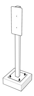
2. Secure the JuiceStand and charging station with the washers and screws.
