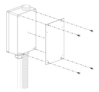
**NOTE:** In the next step, the backplate and charging station are handled as an assembly.
