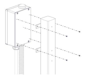
5. Release the fasteners that secure the backplate to the charging station. Remove the backplate.
