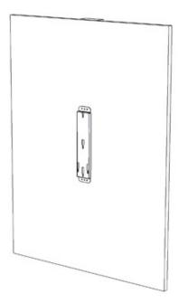
4. Insert the enclosure screws into the enclosure, as shown. Tighten the screws until approximately 2 mm of thread are visible.
